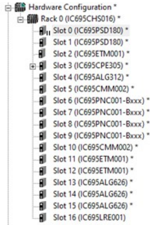
Figure 6: Example of Typical Dual PSD180 System
